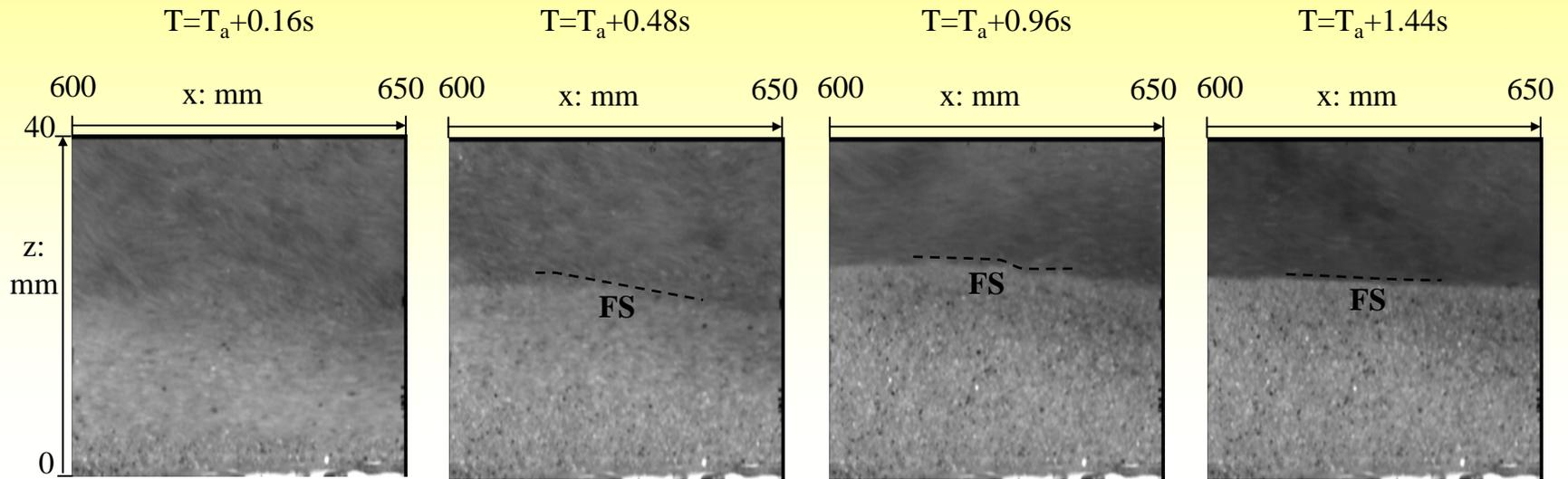
$T_a$ : Instant of time when the flow head arrived at the station of observation ( $x=650\text{mm}$ )
