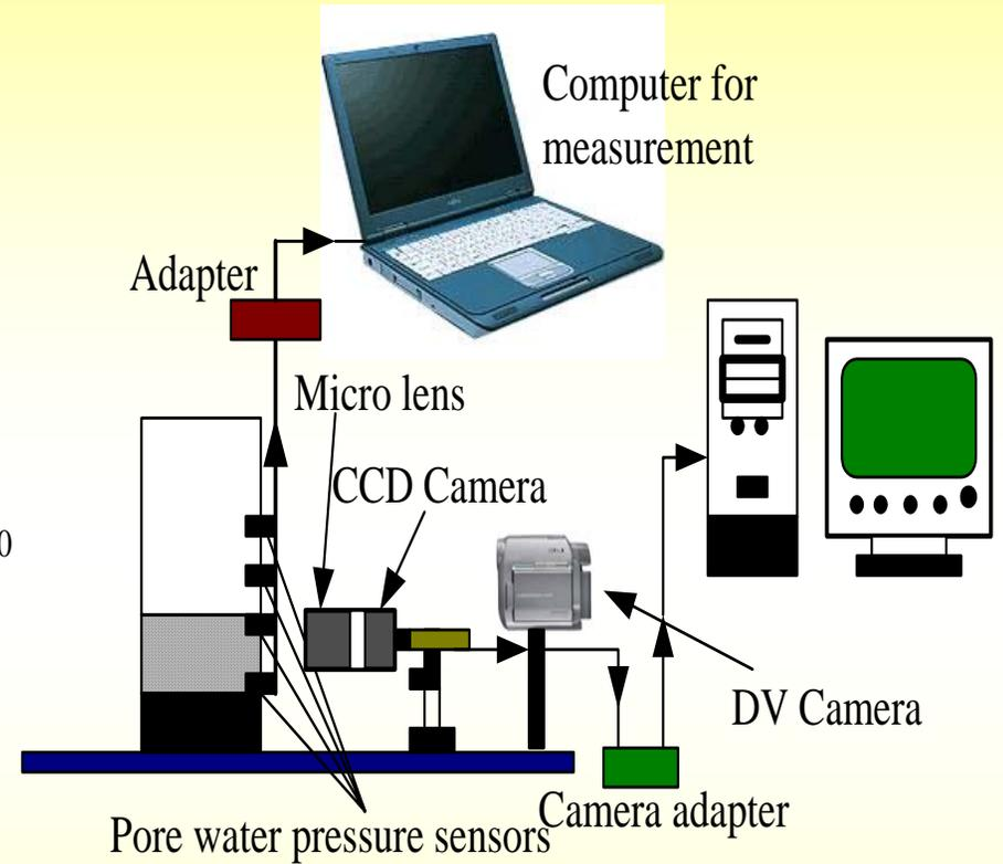
Applications of high-speed CCD and PIV technique
