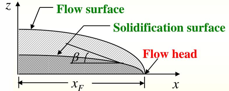
$\beta \leq \beta_{cr} =$  **critical angle in view of frictional resistance of the soil**
