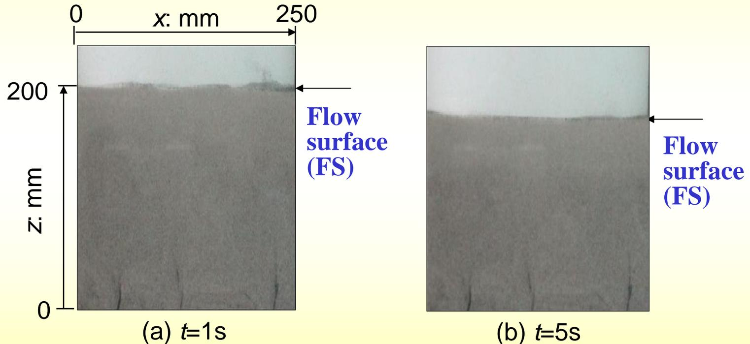
**Identification of the downward advancement of the settling surface following the cessation of fluidization**
