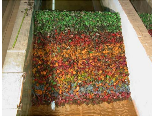
(a) Model Breakwaters in the Twin-flume
