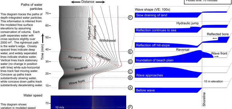
variation in modeled speed (the absolute value of velocity) through time and space. Yellow indicates fast moving water, while blue indicates slow or stationary water. Sharp transitions in velocity (appearing as kinks in the water paths) indicate steps in the water surface. In general I assume that faster water tends to deposit coarser sediment, if it is depositional (see below). Note that this diagram is redundant with the one above, except that it is higher resolution.
